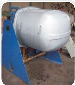
Fresh Water Generator & Spares
